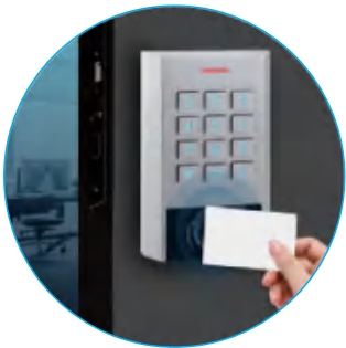
Card type: 13.56MHz Mifare card (4 Byte, 7 Byte ISO14443A Compatible)
